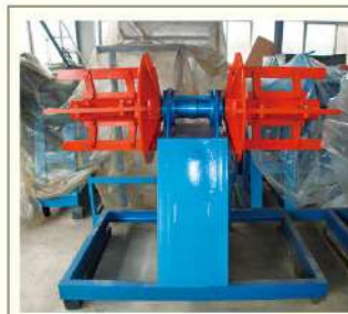
-10 tons simple manual uncoiler -Character: its leaves can be adjusted so that can suit different inner diameter coil (508/610mm)
