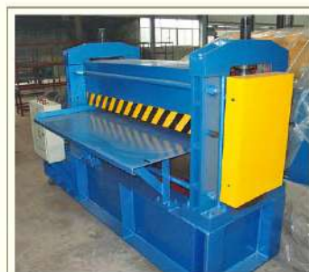
-Aluminum sheet embossing machine -1250mm width, 0.5-0.6mm
