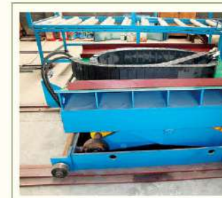
-Character: semi-automatic function and synchronous coordination function with the forming machine or other production line. -We can make hydraulic uncoiler according to the coil's capacity, such as 5tons, 8 tons.
