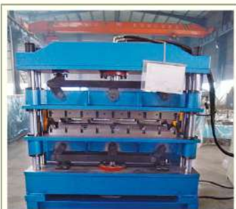
-Hydraulic arching machine -STWYX38-260-1000
