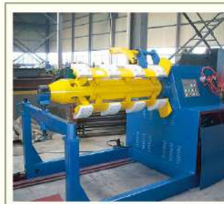
-Character: semi-automatic function and synchronous coordination function with the forming machine or other production line. -We can make hydraulic uncoiler according to the coil's capacity, such as 5tons, 8 tons.
